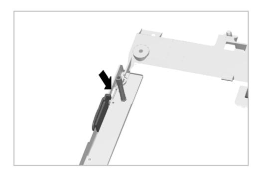
Figure 5-43. Installing the Battery Release Assembly
